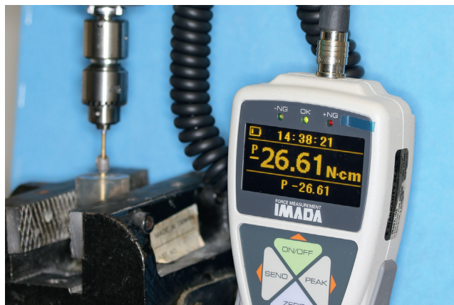
Figure 4. Calibrated digital tightening device.
